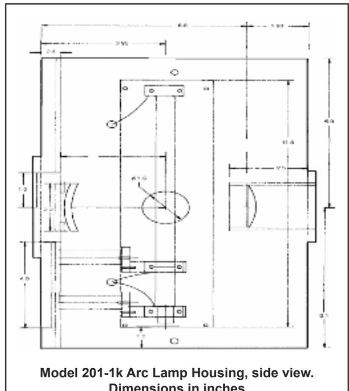
Model 201-1k Arc Lamp Housing, side view. Dimensions in inches.
