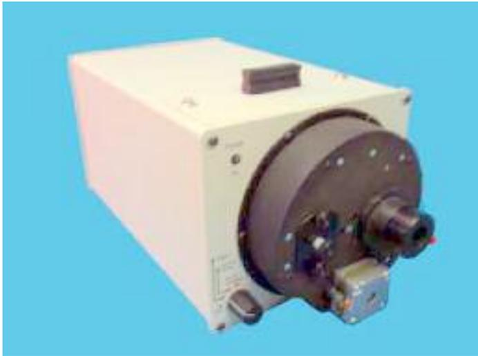
Sciencetech's FB-QTH-3 fibre optic illuminator can fully illuminate a fiber bundle with a diameter up to 13 mm (with appropriate adapter) and a maximum numerical aperture of 0.45 (f/1). A QTH lamp with dichroic elliptical reflector and a folding dichroic mirror allow maximum throughput with very efficient elimination of infrared radiation.
