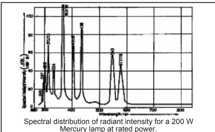
Spectral distribution of radiant intensity for a 200 W Mercury lamp at rated power.
