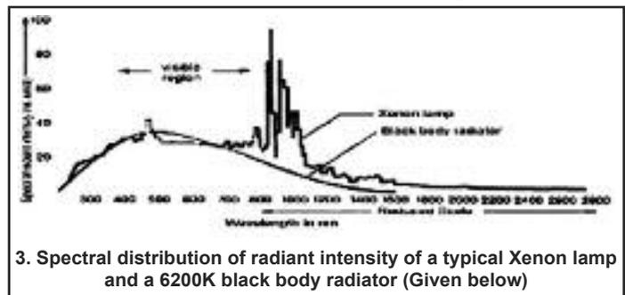
3. Spectral distribution of radiant intensity of a typical Xenon lamp and a 6200K black body radiator (Given below)
