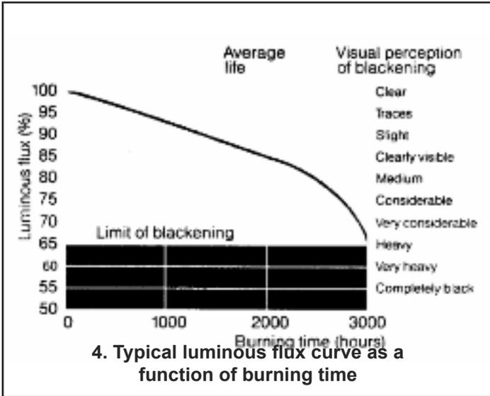
After the average lifetime has been exceeded by 25%, the quartz glass has usually re-crystallized to such an extent that there is an increased risk of bursting.
