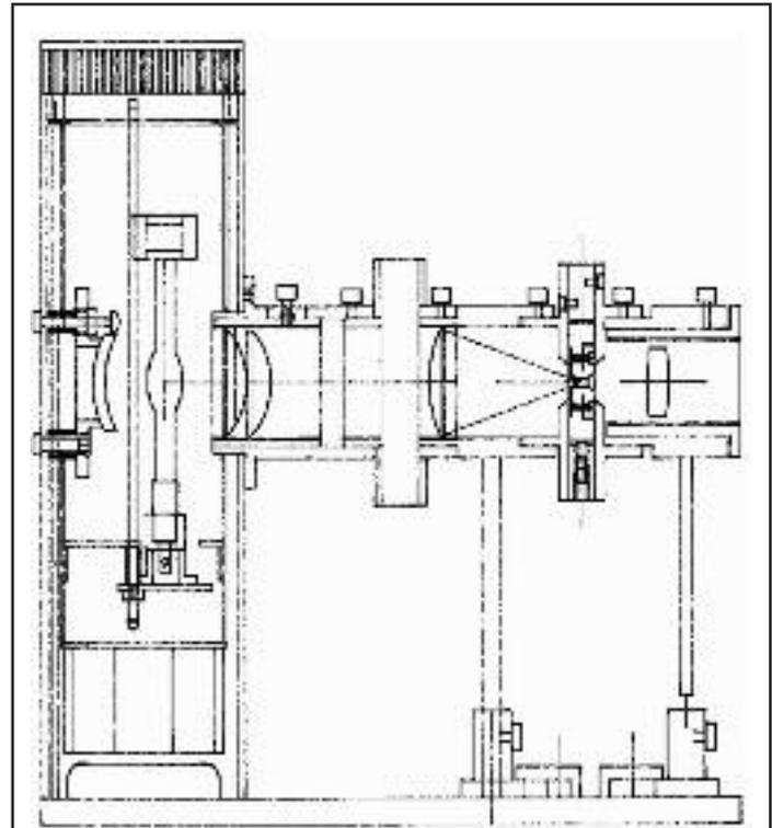
Air Cooled Arc Source model 201-100 with collimator, filter drawer, condenser, and adjustable pinhole
