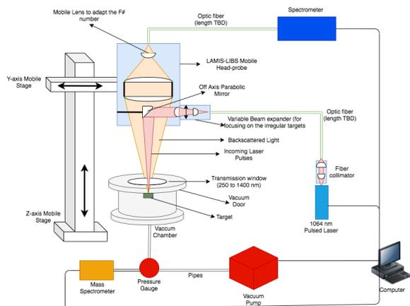
**Figure 1.** Sketched configuration of the LABEISS breadboard system.
