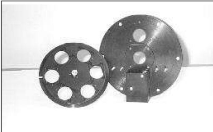
Sciencetech standard filter wheels can hold six, eight or twelve 1" round or square filters up to 5 mm thick. One position is usually supplied with a dark cover for zero referencing. Filters are easy to position and replace. All filter wheels come with a light tight housing. Both manual and motorized models are available.
