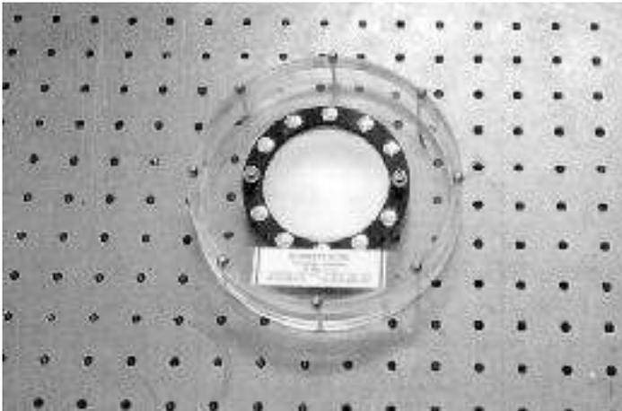
Sciencetech large area far-infrared grid polarizers P280 consist of a conducting grid of parallel wires on a thin substrate. They polarize light for wavelengths longer than the spacing between the wires with a very high degree of polarization.
