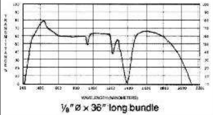
Transmission for Extended Infrared Polymer-clad Quartz Bundles
