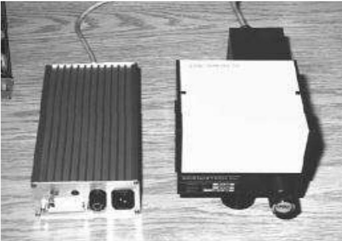
Sciontech model MD-100 motor drive unit and Model 9030 monochromator
