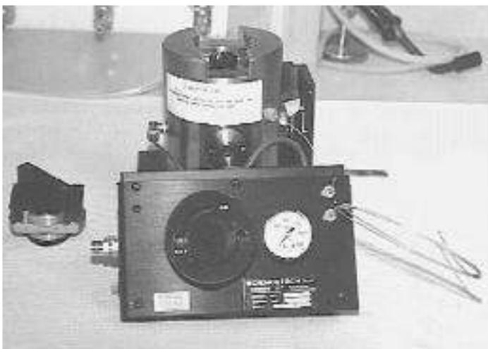
The Sciencetech 3100 hyperbaric cell allows fluorescence and transmission measurement under pressures of up to 200 atm (2x104 kPa, 2900 psi) of liquid samples using a standard 10 mm cuvette. It includes three ports with quartz windows, an excitation port, a 90° port for fluorescence measurements, and the third port for the optional 180° fluorescence/transmission measurements.
