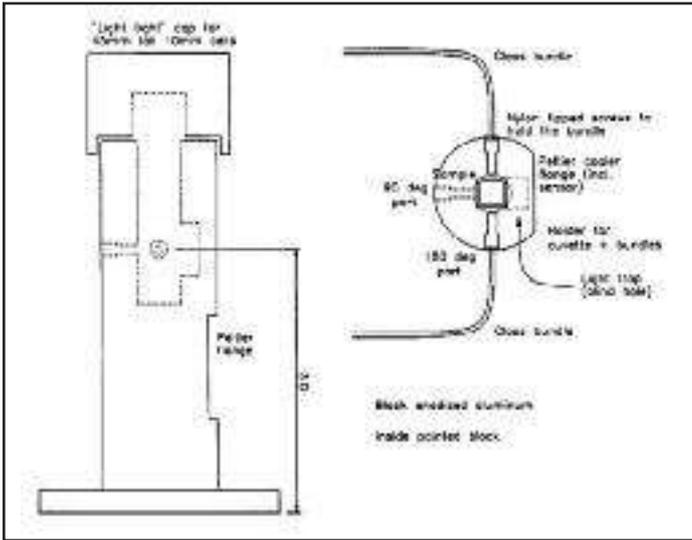
The SC3310 sample chamber allows mounting of standard 10 mm spectrophotometer or fluorescence cells in a light tight configuration (light tight housing not shown in diagram).
