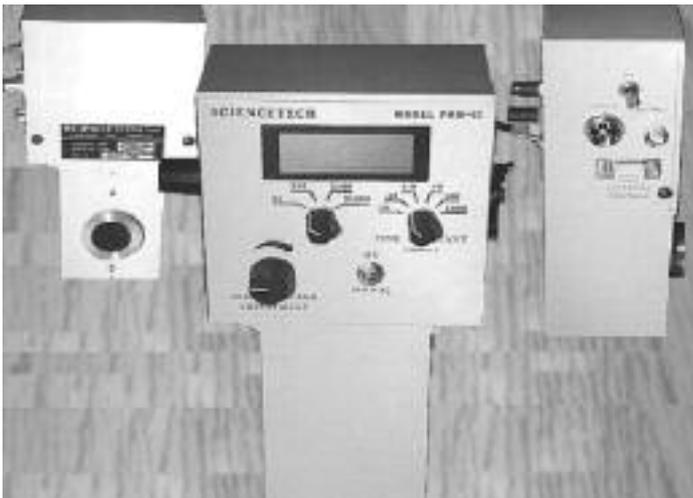
The Sciencetech PMH-02 Photomultiplier housing is a self-contained compact unit for operation of photomultipliers in analog mode. The PMH-02 housing operates at room temperature. The PMH-04 is a Peltier cooled unit (see corresponding brochure).
