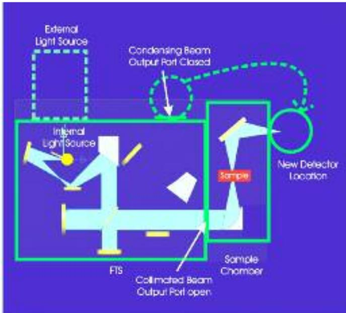
The Model SPS-300 can be used as a terahertz materials transmission and reflectance spectrometer by mounting an external sample chamber to its collimated beam output port. The external terahertz detector would need to be relocated to the detector output port of the sample chamber. In this configuration, either an external terahertz light source or the SPS-300 built-in internal terahertz light source can be used to illuminate the sample.
