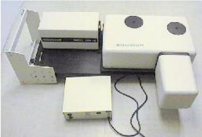
Sciencetech manufactures three models of its ultra-high efficiency solar simulators. The smallest model is the 500W model, which approaches the power output of most conventional 1000W solar simulators on the market. Sciencetech also manufactures 1000W and 1600W models which are also noticeably more intense than competing models of the same power rating.
