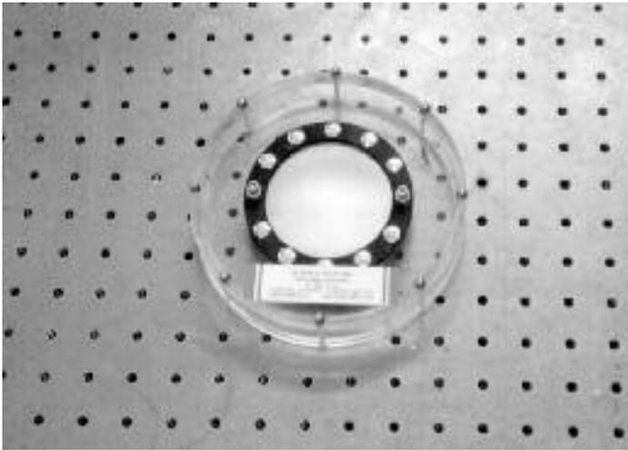
Sciencetech large area far-infrared grid polarizers P280 consist of a conducting grid of parallel wires on a thin substrate. They polarize light for wavelengths longer than the spacing between the wires with a very high degree of polarization.
