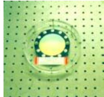
set by the grid separation of 4 $\mu$ m. The Model SPS-300 also features large 90mm optics for high light throughput, a high precision translating stage, large roof mirrors, and large input/output off axis paraboloids to support a 4" diameter output beam.
