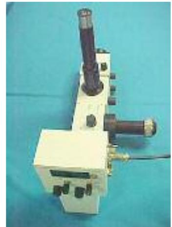
*MPT-8000 shown with Sciencetech PMH-2 PMT Detector attached*
