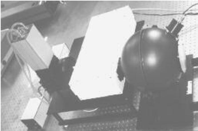
Sciencetech offers complete modular spectroradiometric systems which include a Sciencetech light source, automatic monochromator, filter wheel and calibrated detector. The systems are fully integrated and calibrated, featuring very high light throughput and minimal stray light.
